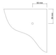
It is necessary to design the hole size in order to allow the thermal dilatation of the aluminium profiles without generate tensions on the slab.
